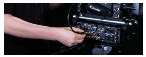
If you have a camcorder with an HDMI output, it can also provide audio and video - but not timecode - with one single cable to Ki Pro.
