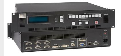
The DCS-100 is a dual-channel switcher designed to provide true seamless switching between different input sources and formats, while maintaining superb scaling quality at an affordable price. It has been designed for straightforward and simple operations, which makes it the ideal seamless switcher for live events, boardrooms, hotel ballrooms, houses of worship, lecture halls, training facilities and more.
