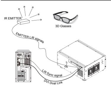
Connect the STEREO DVI to a stereo 3D source – it is usually a computer with 3D Graphics card, and 3D applications.
