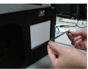
3. Reattach the filter cover and tighten the two screws.
