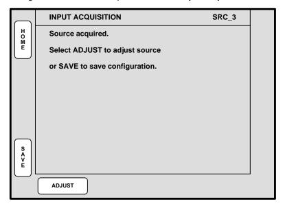
Figure 4-4. Input Acquisition Menu: No File Saved (sample)
