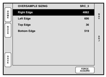
Figure 4-8. Oversample Sizing Menu (sample)
