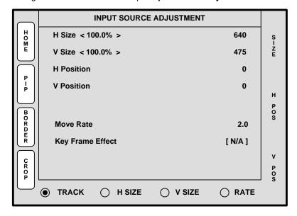
Figure 4-41. Input Source Adjustment Menu (sample)
