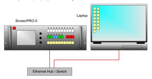
Figure C-4. Small Ethernet Network
