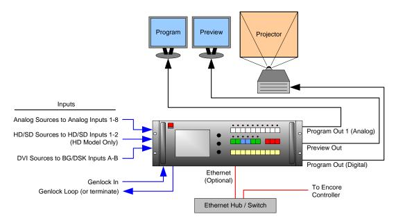
Figure 3-1. Block Diagram, Basic ScreenPRO-II System
