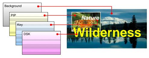
Figure 1-2. Layer Illustration — Background, Mixer and DSK
