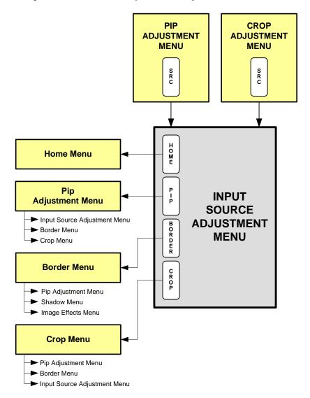
Figure 4-40. Input Source Adjustment Menu Tree
