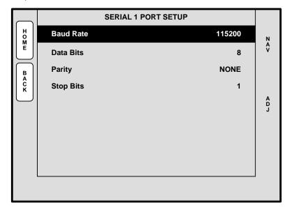
Figure 4-23. Serial 1 Port Setup Menu (sample)
