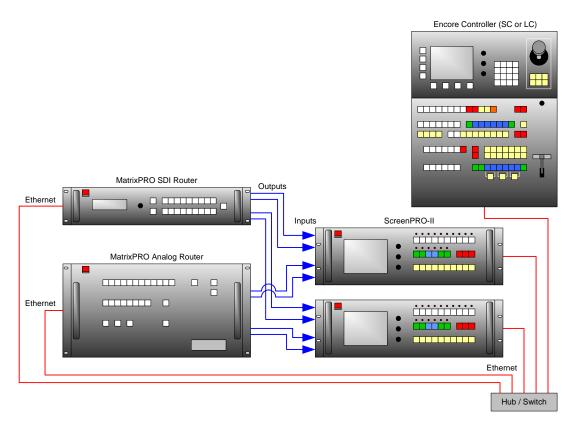
Figure D-3. ScreenPRO-II Units using External Ethernet Controlled Routers
