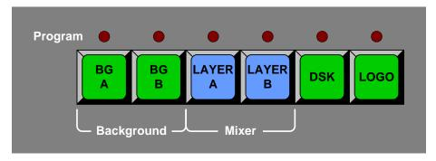
Figure 2-5. Layer Control Section
