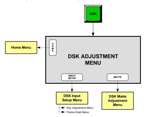
Figure 4-47. DSK Adjustment Menu Tree
