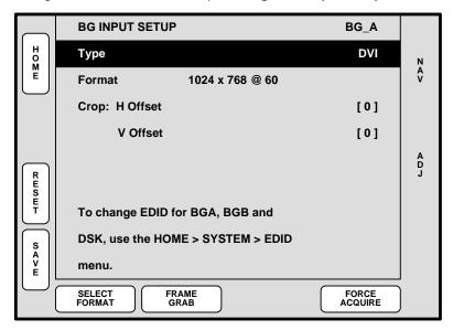
Figure 4-43. Background Input Setup Menu (sample)
