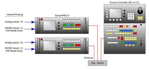
Figure D-1. ScreenPRO-II Units using Internal Source Routing
