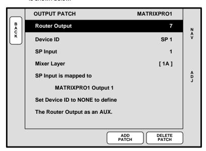
Figure D-9. Output Patch Menu (sample)
