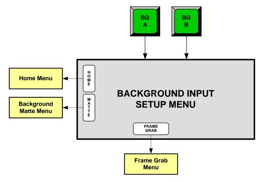
Figure 4-42. Background Input Setup Menu Tree
