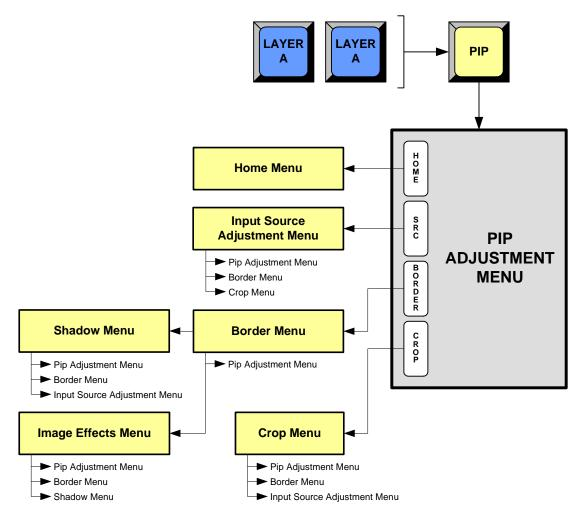
Figure 4-30. PIP Adjustment Menu Tree
