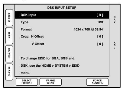
Figure 4-49. DSK Input Setup Menu (sample)
