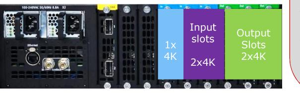
For both E2 and S3-4K all output slots support 2x 4K60 when using Gen 2 cards
