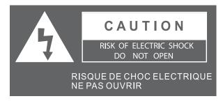
The lightning flash with arrowhead symbol within an equilateral triangle, is intended to alert the user to the presence of uninsulated. "Dangerous Voltage" within the products enclosure that may be of sufficient magnitude to consitute a risk of electric shock to persons.
