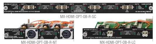
MX-HDMI-3D-0B-R is an eight channel Multimode optical Output Board providing HDMI 1.4, audio and RS-232 extension over a single Multimode fiber up to 2500m distance. Pixel Accurate Reclocking, HDCP compliance and HDMI to DVI conversion are incorporated. Resolutions up to 4K and 36-bit color depth are handled with all standard audio formats as well as 120Hz 3D signals.
