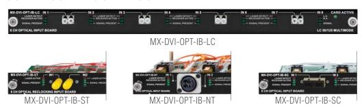
MX-DVI-OPT-IB offers an extremely long, 2500m distance extension over a single Multimode fiber for Single-Link DVI signals on eight channels. The board is available with Neutrik OpticalCON, -LC, -SC or -ST connectors. Each port converts an incoming fiber signal to DVI-D format. Single Fiber Technology ensures transmission of DVI-D signals over one multimode fiber core using multiple wavelengths.
