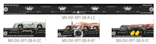
MX-DVI-OPT-OB-R Output Board provides extremely long, 2500m extension and reclocking for DVI-D signals over Multimode fiber on eight channels. It incorporates our Pixel Accurate Reclocking technology and Single Fiber Technology. Fiber connectors are available with Neutrik OpticalCON, -LC, -SC or -ST connectors.
