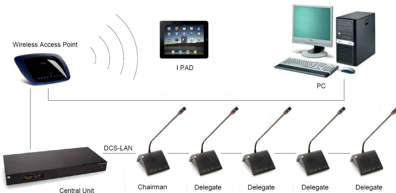
Figure 10. Connecting the DDS 5900 Digital Discussion System to a PC and an iPad
