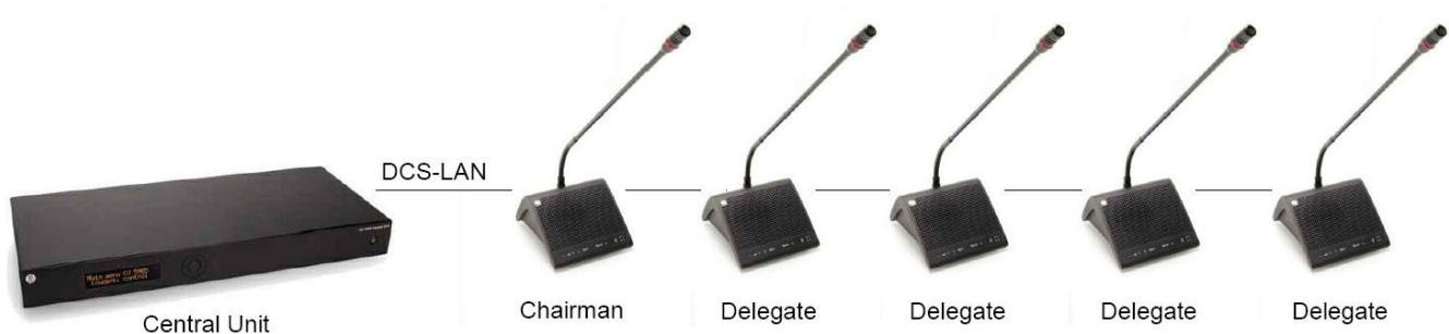
Figure 8. Connecting the DDS 5900 Digital Discussion System.
