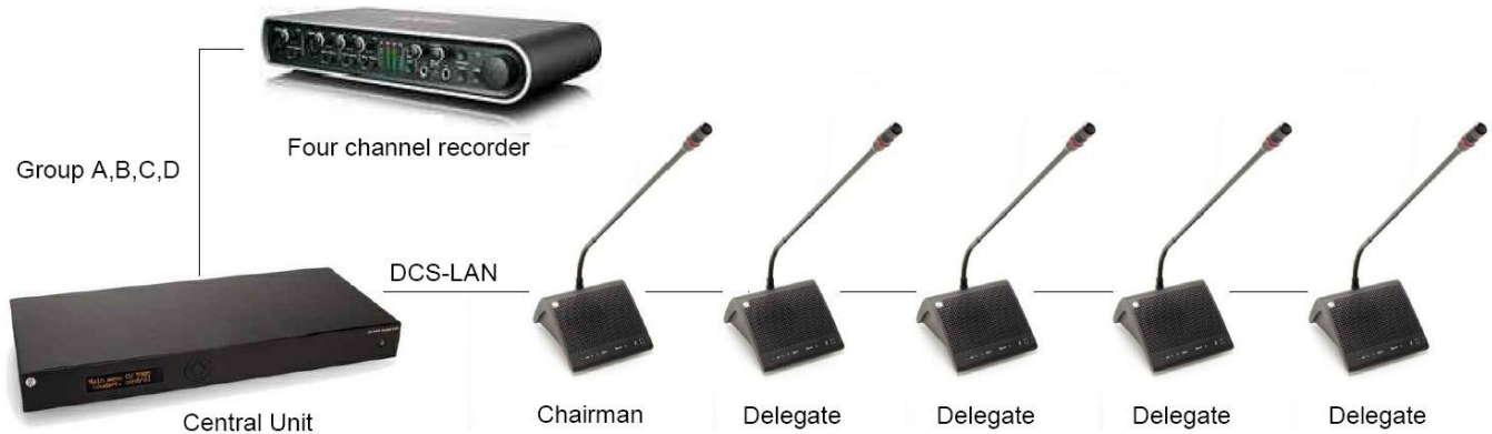
Figure 11. Connecting the DDS 5900 Digital Discussion System to an Audio Recorder.
