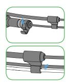
Unclip the boom from the two clips along the back of the headset.
