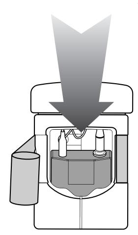
Afterwards, place the 3rd party transmitter inside the cavity of the Catchbox Pro Module, making sure no antennas or cables are protruding outwards.
