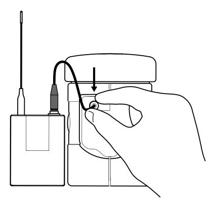
Place the transmitter inside the cavity of the Catchbox Pro Module making sure no antennas or cables are protruding outwards.
