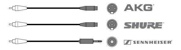
Choose an adapter cable based on the brand and model of your 3rd party transmitter and connect it to the microphone input of said transmitter.
