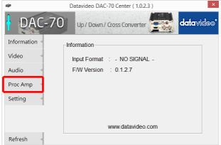
Set the Brightness, Contrast, Hue, and Saturation levels on the Proc Amp setup page.
