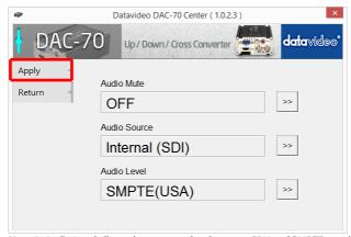
**Note 1**: Audio Level allows the user to select between EBU and SMPTE standards. **Note 2**: Audio Level setting is enabled only for RCA input.
