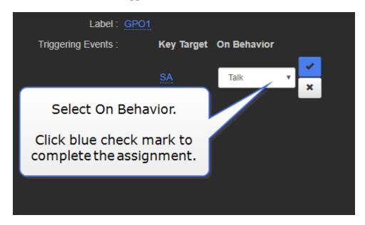
In this example, where the target is set to **Stage Announce**, and the behavior is set to **Talk**, an output trigger is sent whenever the Stage Announce button on the Base is pressed. This replicates existing functionality, but the GPOs can be set to any configuration you require. You can set up to 10 actions on each GPO.
