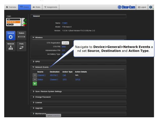
1. Configure trigger for an FOR22 radio (example)
