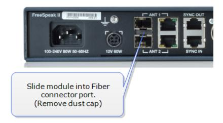
Install splitter Fiber module.
