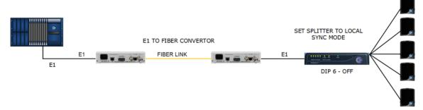
The transceiver connections are switched between RJ45 and Fiber routing using dip switches set inside the splitter.
