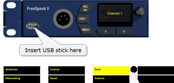
Press Menu key. Navigate using rotary controllers.
