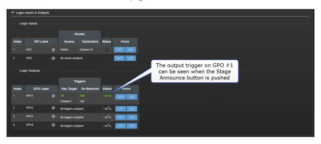
Note: Each GPO can be used to generate up to 10 different actions.
