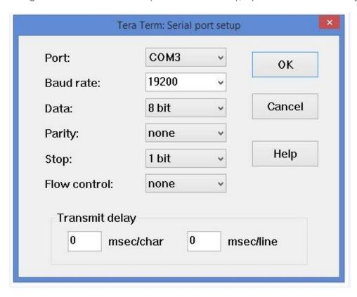
5. Open the serial console. Press the space bar and the splitter will output its software version as shown.
