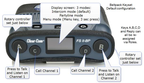
To navigate through menu use either controller. In menu mode, key C to go back, key D to select or commit. Rotary controllers also control beltpack volume.
