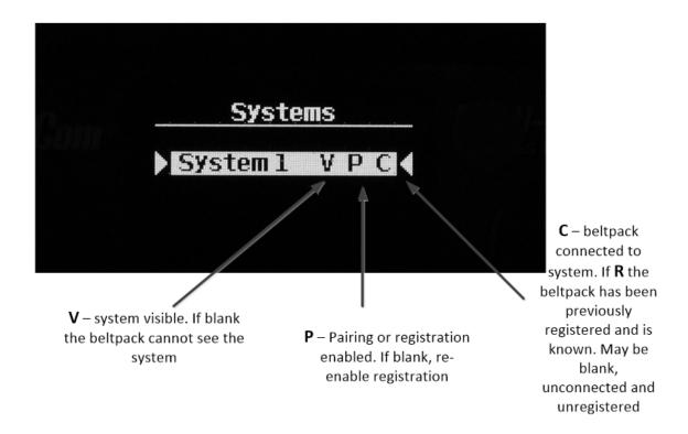
Connect the beltpack to the system using key D.
