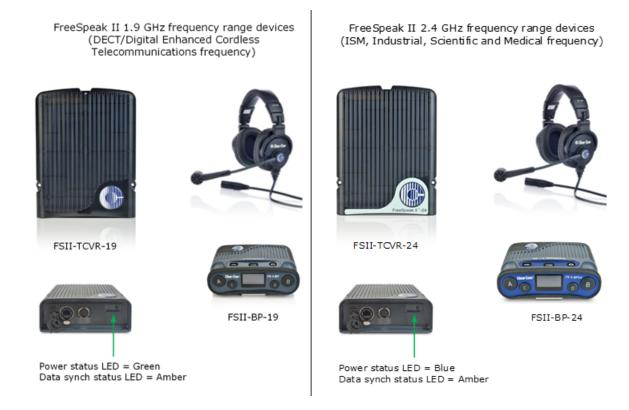
The two sets of equipment can be used separately or together.
