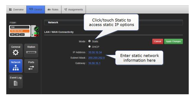
Set static IP address from the Base Station menu screens.
