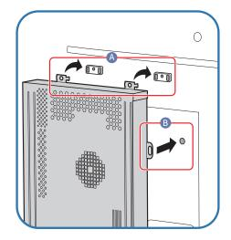
2 First insert the tabs of the network box into the slots marked (A) on the attachment frame. The tabs should hook onto the frame. Then, align the holes marked (B).
