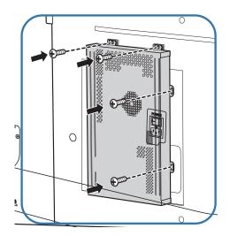
Attach the network box to the fixed attachment frames.
