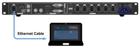
Scenario 2: MCTRL660 PRO connected to PC (or mobile device) via LAN
