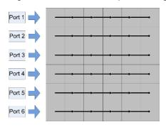
Figure 7-9 Each Ethernet port loading only one column of cabinets
