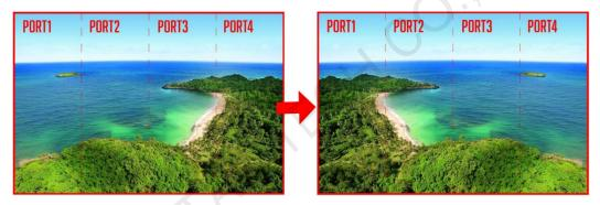
As shown above, after you set the mirroring mode as left-right for Ethernet ports 1-4, the entire image is mirrored horizontally.
