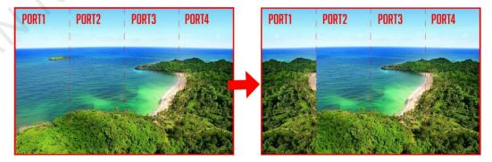
As shown above, after you set the mirroring mode as left-right for Ethernet port 1, the entire image is mirrored horizontally, but only the Ethernet port 1 area displays the partial mirrored image.
