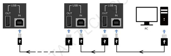
Multiple MCTRL660 PRO devices need to output image simultaneously.
