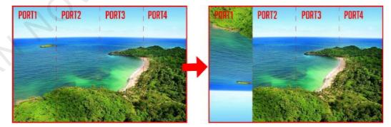
As shown above, after you set the mirroring mode as top-bottom for Ethernet port 1, the entire image is mirrored vertically, but only the Ethernet port 1 area displays the partial mirrored image.
