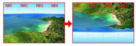
As shown above, after you set the mirroring mode as top-bottom for Ethernet ports 1-4, the entire image is mirrored vertically.
