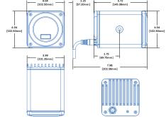
Dimensions 4.04" w x 4.04" h x 5.72" (7.98" with connector) d (102.50 mm x 105.50 mm x 145.38/202.58 mm)
