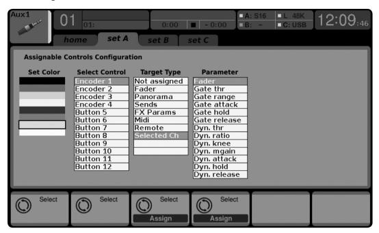
The "Set A" tab allows mapping of specific console parameters to the 8 assignable buttons and 4 assignable rotary encoders. Using this screen, the user can map the exact parameters that are most useful to them to the desired controls, in the desired order.
