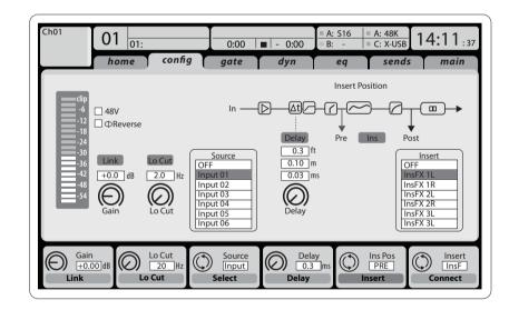
**Input Channels 1-32** are pre-configured to use the first 32 input signals, but can be patched to use any other available signal on the audio engine as well, including mix bus/sub group outputs. Changes of the Channel Source can be made on the Preamp Config page.
