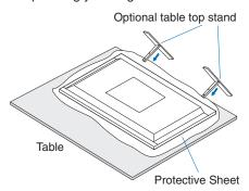
NOTE: Install the stand in the direction of the arrow which is imprinted on the surface of the stand.
