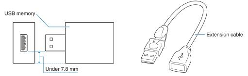
**NOTE:** If the monitor does not recognize a connected USB storage device, make sure the file structure is FAT32 or FAT16. It is not guaranteed to work with all USB memories sold commercially.
