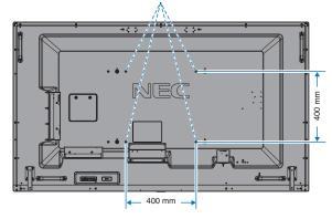
Mounting accessories can be attached with the monitor in the face down position. To avoid scratching the LCD panel, always place a soft cloth, such as a blanket that is larger than the monitor's screen area, on the table before laying the monitor face down. Make sure there is nothing on the table that can damage the monitor.
