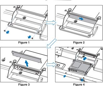
4. Insert the Option Board into the monitor and fix it with the removed screws (Figure 4).
