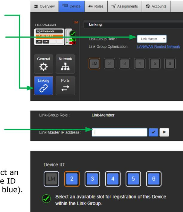
**Note:** For Link-Groups that include HelixNet, you must designate the HelixNet Main Station as the Link-Master, and link LQs to it as described above.
