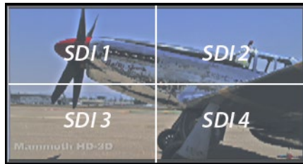
Figure 6. Mapping of Quad SDI Outputs
