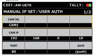
3. Set the IP address (remote camera) and PORT number.
