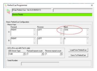
When the user presses the Blank button on the transmitter, and Port A is connected to the MAC, the application will receive "[Command] b"
