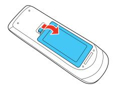
2. Insert the batteries with the + and – ends facing as shown.
