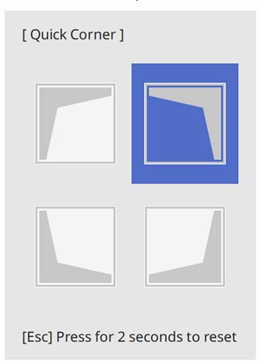
6. Use the arrow buttons on the projector or remote control to select the corner of the image you want to adjust. Then press - Enter.
