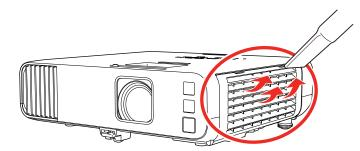
**Note:** You can remove the air filter so you can clean both sides of it. Do not rinse the air filter in water or use any detergent or solvent to clean it.
