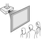
You can mount the projector to the ceiling at any horizontal or vertical angle.
