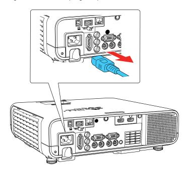
**Caution:** To avoid damaging the projector or laser, never unplug the power cord when the Status light is on or flashing.
