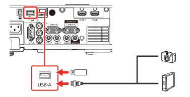
**Note:** Use the USB cable supplied with or specified for use with your device. Do not connect a USB hub or a USB cable longer than 10 feet (3 m), or the device may not operate correctly.
