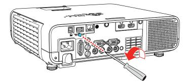
2. Insert the wireless LAN module into a USB-A port.
