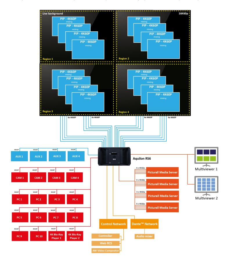
Aquilon RS6 can drive a 16K60p LED wall with up to 16x 4K mixing layers and four 4K60p AUX outputs
