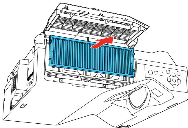
5. Vacuum the front of the air filter (the side with the tabs) to remove any remaining dust.
