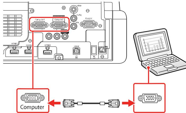
4. Tighten the screws on the VGA connector.
