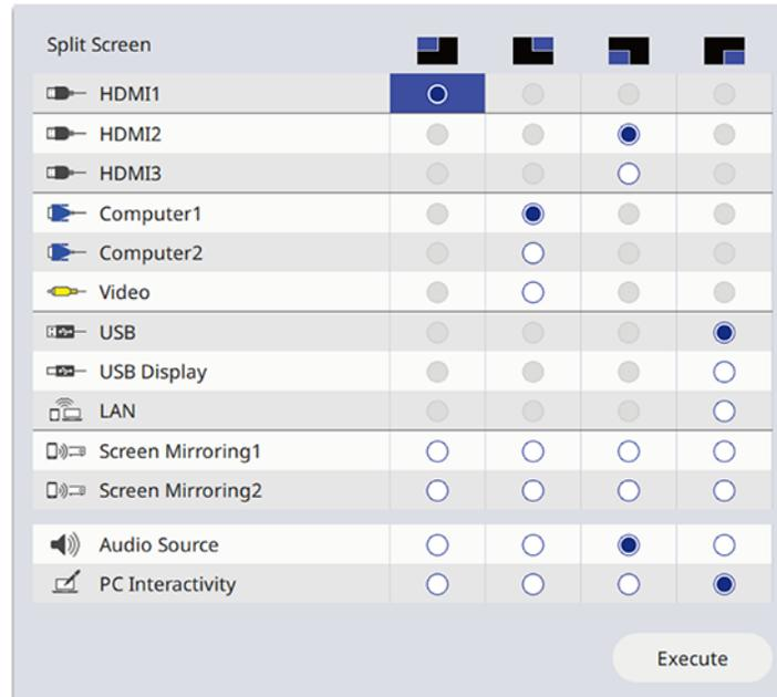
4. Press the arrow and **↵ Enter** buttons to select an image source for each section of the screen.
