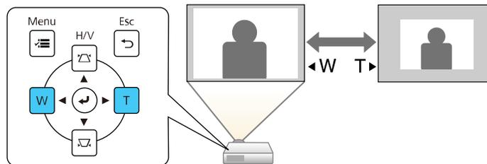
After you adjust the image size, the Image Shift screen is displayed automatically for adjusting the image position.
