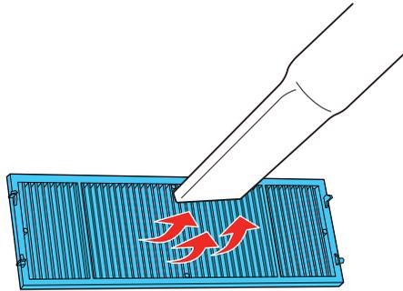
**Caution:** Do not rinse the air filter in water, or use any detergent or solvent to clean it. Do not use canned air; the gases may leave a flammable residue, or push dust and debris into the projector's optics or other sensitive areas.
