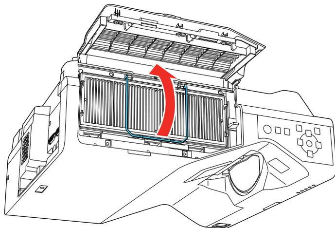
4. Pull the air filter out of the projector.
