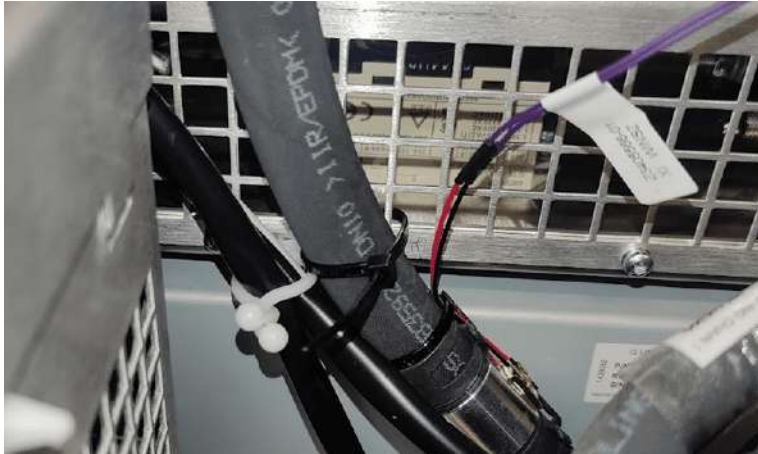
Image 12-44 Example of strapping the tube to the filter cage
