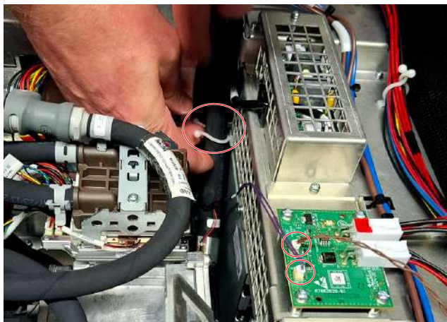
Image 12-43 Tubing and sensor connections on the cooler interconnection board
