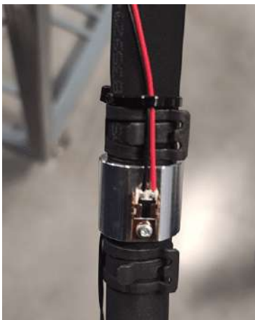
Image 12-39 Desired location to lock the dew point sensor in place
