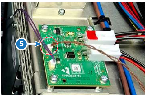
Image 12-33 Location of the two-pin cable on the interconnection board
