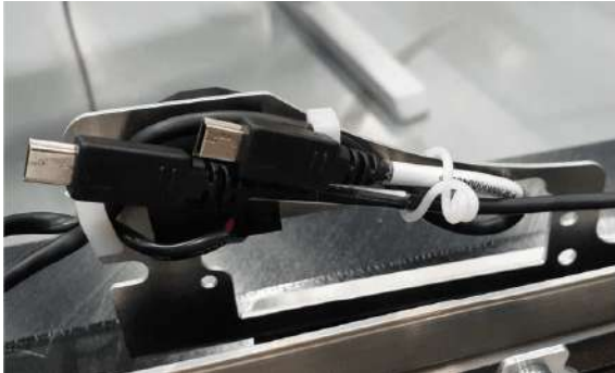
Image 9-14 Mini-USB cables connected to the front bracket
