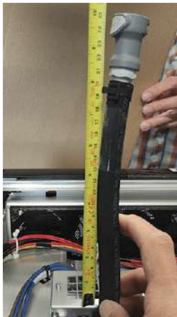
Image 12-45 Example of measuring the length of the tube.
