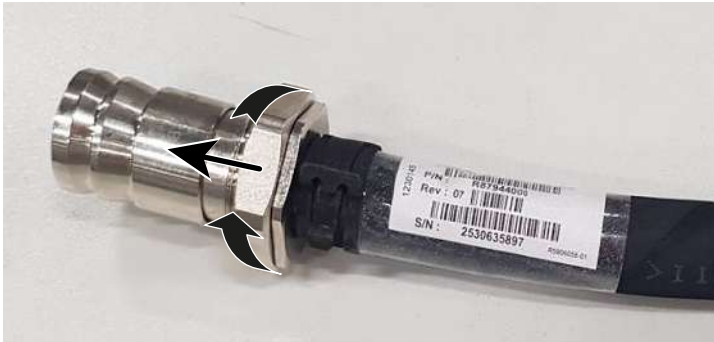
Image 12-38 Remove the lock nut by rotating it counterclockwise
