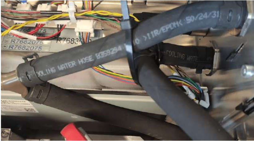
Image 12-47 Example of where to lock the tubes together
