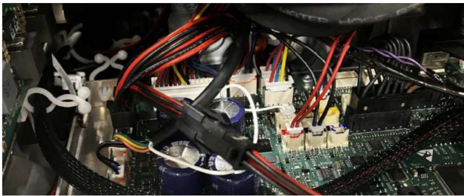
Image 12–14 Location of the wiring on the LCB
