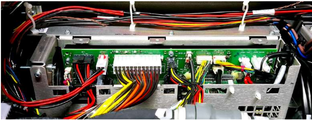
Image 12-22 4-pin cable inserted into the SMPS
