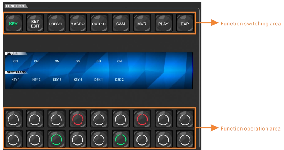
Figure 5-9 Comprehensive control area
